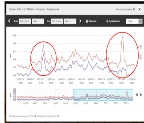
Leak detection using AMR data
